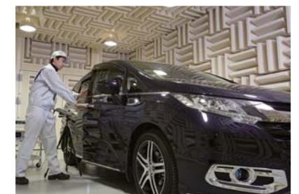
Testing using psychoacoustic technology to monitor the closing sound of car doors in an anechoic room (Mitsui Kinzoku ACT)
